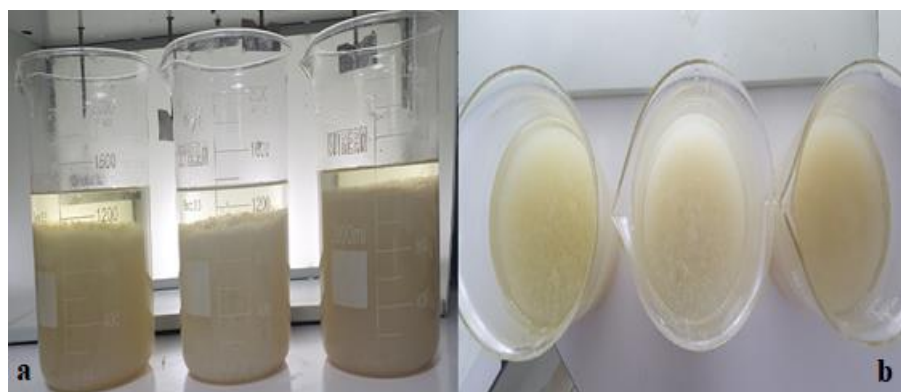
Figure 2. a) Flocculation profile image studied with Modified Starch in pH 5.5 – 7 and 8.5 media, respectively b) Flocculation profile image studied with Modified Starch in pH 5.5 – 7 and 8.5 media, respectively
