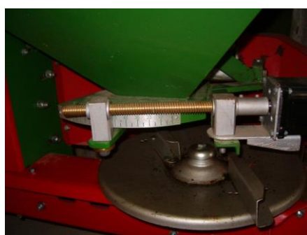
Figure 4. Variable rate controller for centrifugal fertiliser spreader
