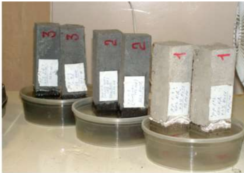
Fig. 1. Salt efflorescence formation on the surface of the samples.
